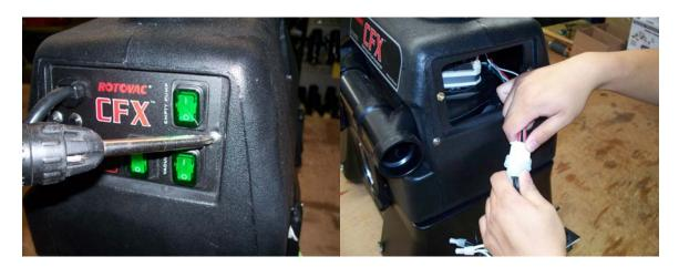
2) Remove the exhaust manifold screw and remove the exhaust manifold.
