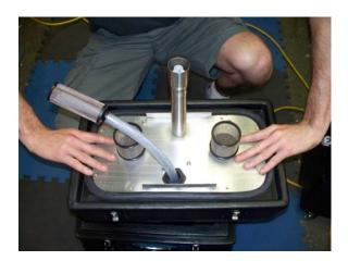
6) Lift up on the top housing, removing it from the deck plate.
